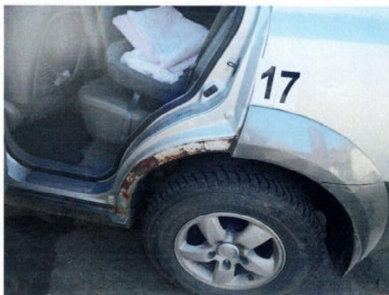
ST 17/25 KIA Sorento JC – detail koroze
